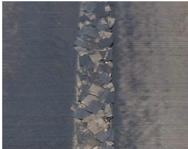
Fig. 5. Underside view of the chopped UD filler before the assembly of the overlaminates and the skin
