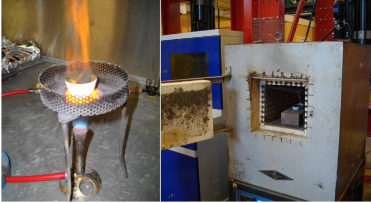
Figure 5 The sample was ignited using a Bunsen Burner (left), and then later placed into a muffle furnace (right)
