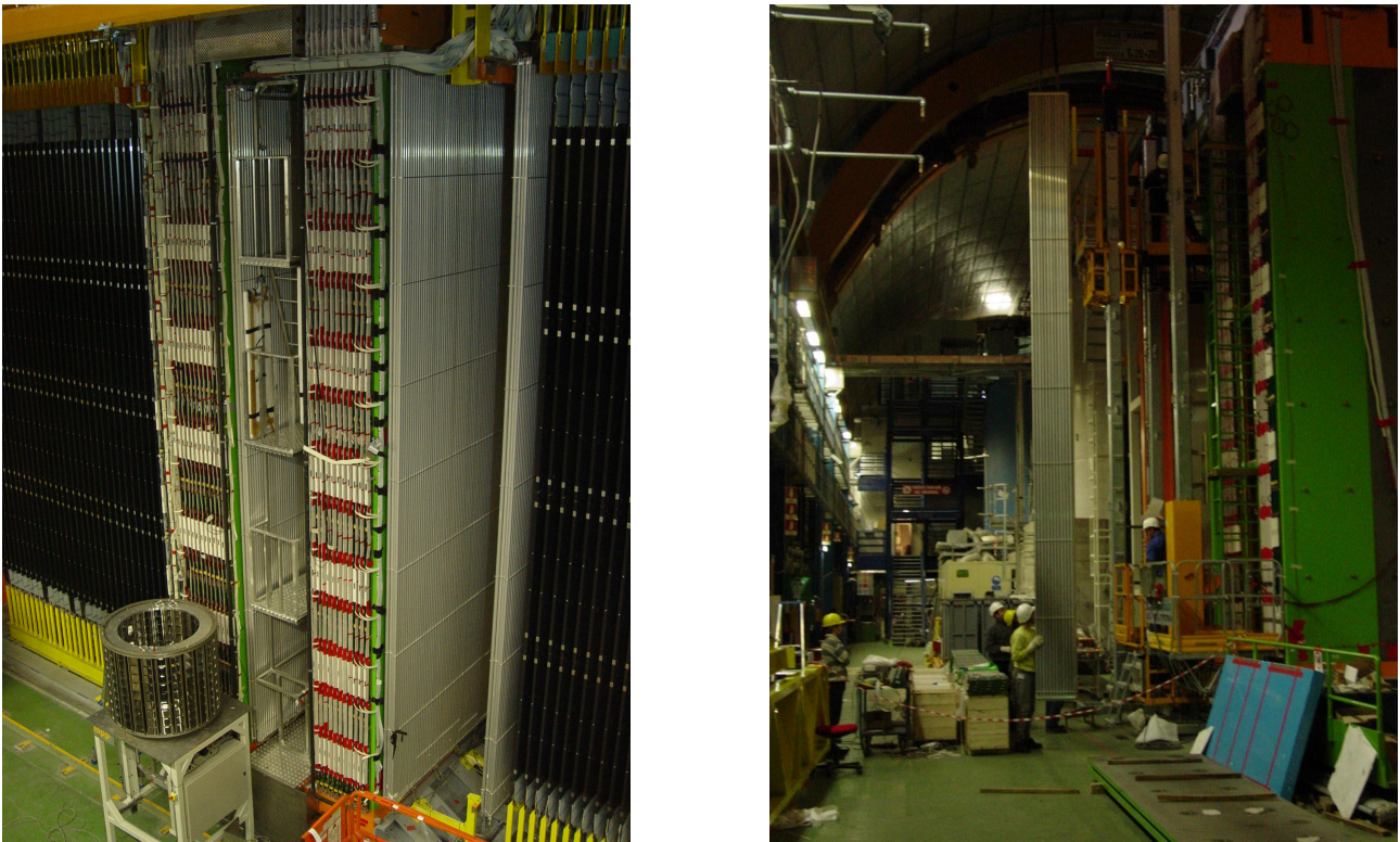
Figure 4.33: (Left) Photograph of the current setup of the drift-tubes in the spectrometer of OPERA. (Right) Installation of a drift-tube module in OPERA
