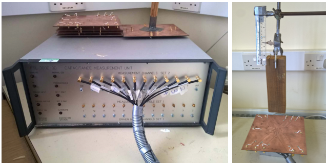
Fig. 5: PTL 300E device for capturing capacitance data and experimental setup.
