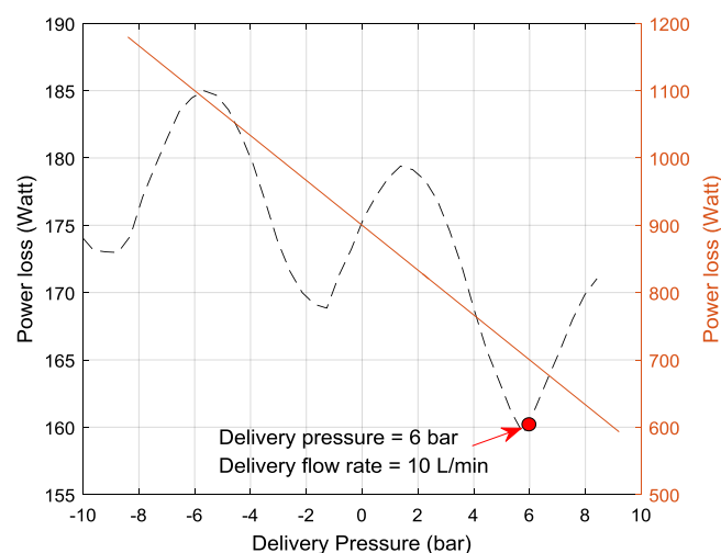
Figure 12. Comparison of power losses between an SIHS and a conventional valve controlled system.
