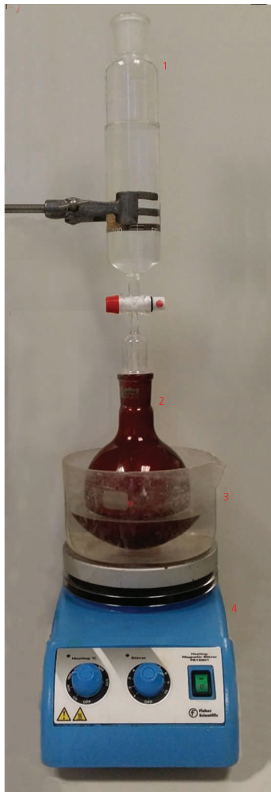
Figure 1. Sol-gel reaction system. 1, separator funnel containing 250 ml of a solution 7 \times 10^{-4} M of cobalt (II) chloride (aq); 21 2, round-bottomed flask containing 2-propanol and the titanium precursor; 3, crystalliser plate with water for the temperature bath; 4, hotplate/magnetic stirrer
