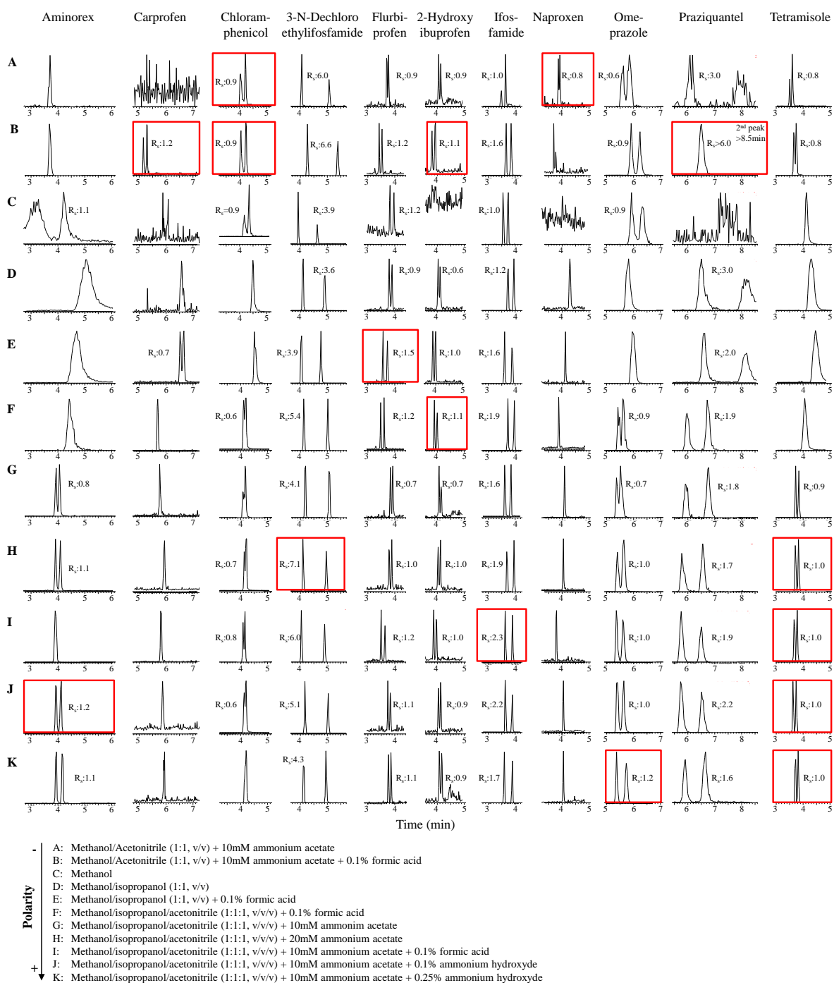
Fig. S3. Effects of mobile phase composition on the enantioseparation of several cPACs in AMY (chromatographic conditions: mobile phase: CO 2 (A')/co-solvent (A-K) (B'); gradient: 0 min – 95 % A', 1 min – 95 % A', 6 min – 40 % A', 8.5 min – 40% A', 8.7 min – 95 % A', 10 min – 95% A'; flow: 1.5 mL/min; ABPR: 1800psi; make-up flow: methanol (0.1% formic acid) for positive ionization and methanol (0.2% ammonium hydroxyde) for negative ionization at 0.3 mL min -1 )
