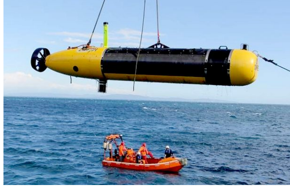
Fig. 3. The MUSCLE autonomous underwater vehicle of the NATO Centre for Maritime Research and Experimentation.
