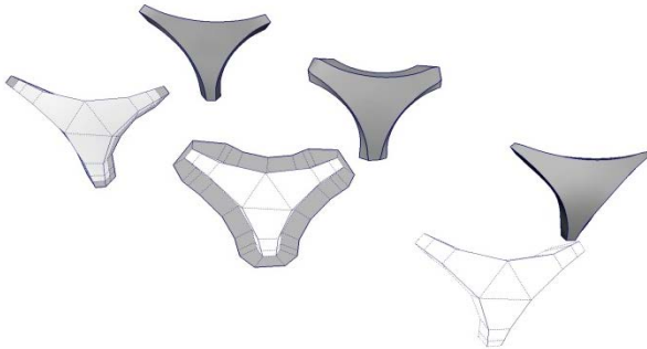
Figure 9 shows three variants of adding extra faces – in plane, extrude normally out and normally in and the resulting equilibrium meshes
