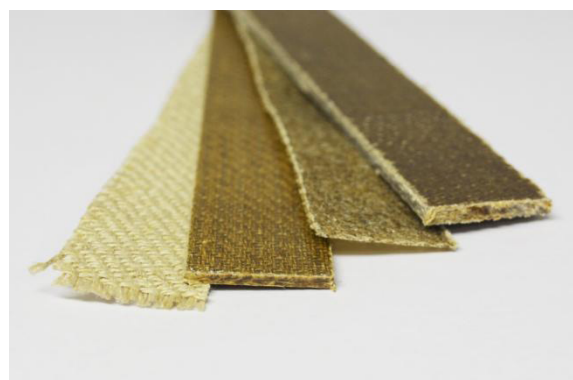
FIGURE 3. Untreated Flax and Flax In Polyamide (left) Coating And The Corresponding Test Specimen (right) Photo By Fraunhofer WKI and Natalie Vellguth 2020
