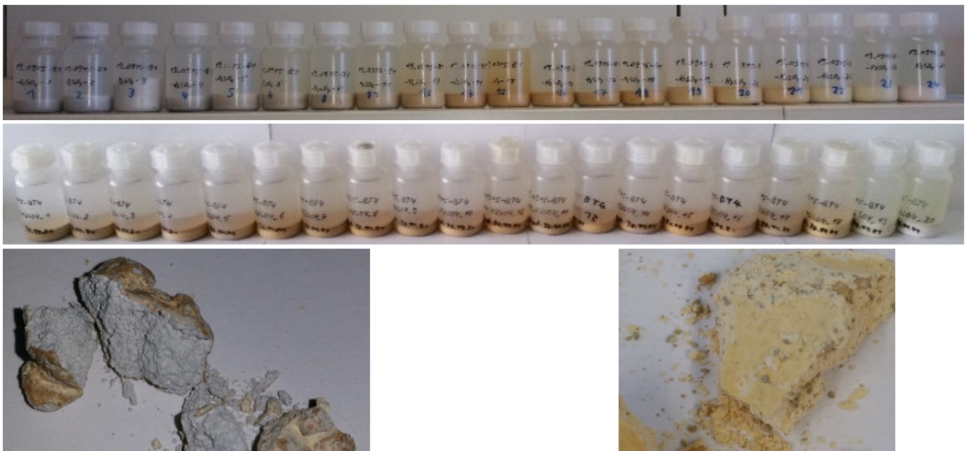
Figure 2 Photographs of selected suspensions before filtration and of the solids after filtration for PC (up) and PC+SF (middle): for each series with decreasing pH from left to right. Some of the solid fractions after filtration for PC with 6.36 mM H 2 SO 4 per g HCP (down, left) and PC+SF with 2.932 mM H 2 SO 4 per g HCP (down, right)
