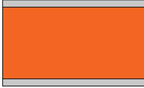
Figure 5.1.: Preliminary 2D simulation model design with BST (orange) between two silver electrodes (gray) without the inclusions. The BST is 2 \times 1 \text{ mm}^2 in dimensions.
