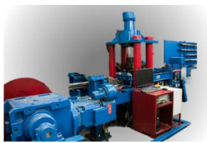
Figure 2. Flat-bed strip draw test, PtU Darmstadt, Darmstadt, Germany [3]
