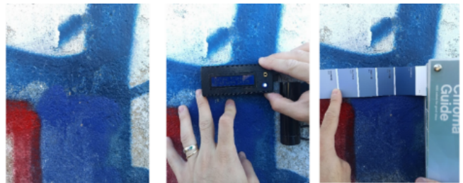
Fig. 17. Comparative study of the data obtained with the sensor and the color chart (graffiti 1) (Redmi Note 8 Pro, Xiaomi f/1.89, 1/168, ISO100, 5.43mm, without Flash) (Redmi Note 8 Pro, Xiaomi f/1.89, 1/162, ISO100, 5.43mm, without Flash).
