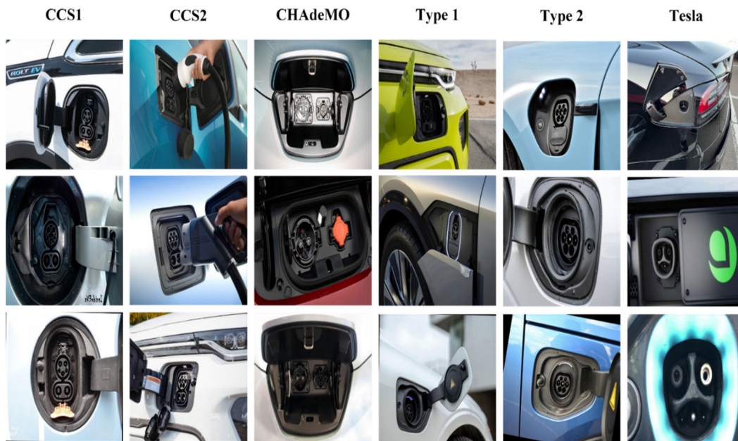
FIGURE 7. A Representation of different classes of EV sockets present in the dataset [18].
