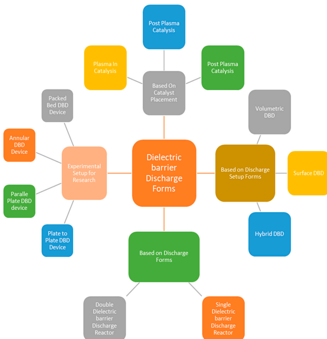
Figure 1. Discharge barrier NTP technology characteristics for gasification tar reduction, based on [44].
