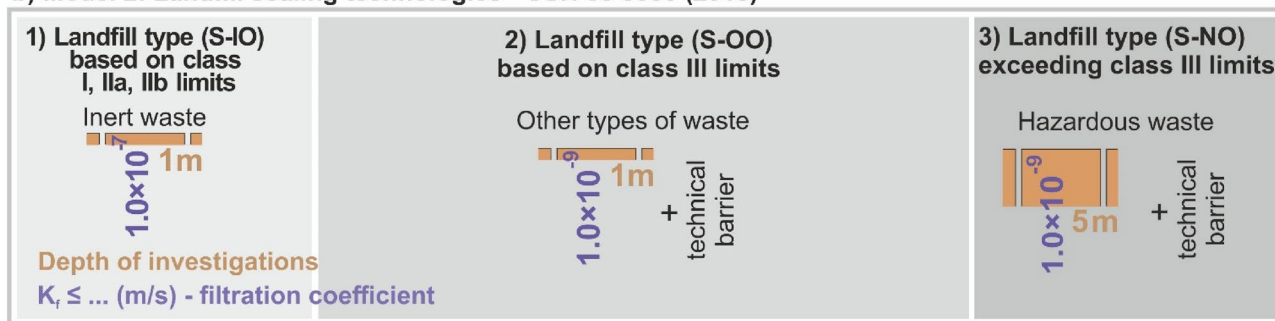
Figure 1. Requirements for the landfill’s geological subsoil (two parameters—the depth of the engineering-geological investigation, and the impermeability of the geological environment based on filtration coefficient) in the sense of the geological barrier for the disposal of waste based on landfill categories and the limit leachability values (Table 1); (a) Model 1 according to CSN 83 8030 49 Standard, (b) Model 2 according to CSN 83 8030 50 Standard.
