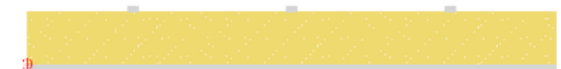
Figure 54. Layout of the 100 mm, 76 mm and 33 mm Long Microstrips. The bottom side is completely covered with the ink. The depiction of the cross section is not to scale.
