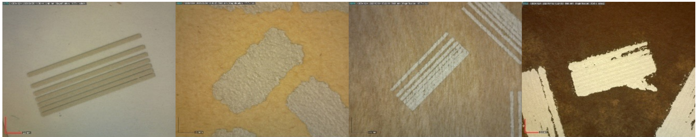
Figure 22. Screen printed silver paste patterns on uncoated substrates for fire retardant coating. From up to down, PET ref., PankaMax, KoskiPly veneer and Palonot FI-00 coating.
