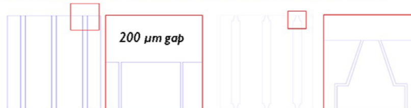
Figure 55. Layout, Cross Section and End Detail of a Coplanar Waveguide Structure.
