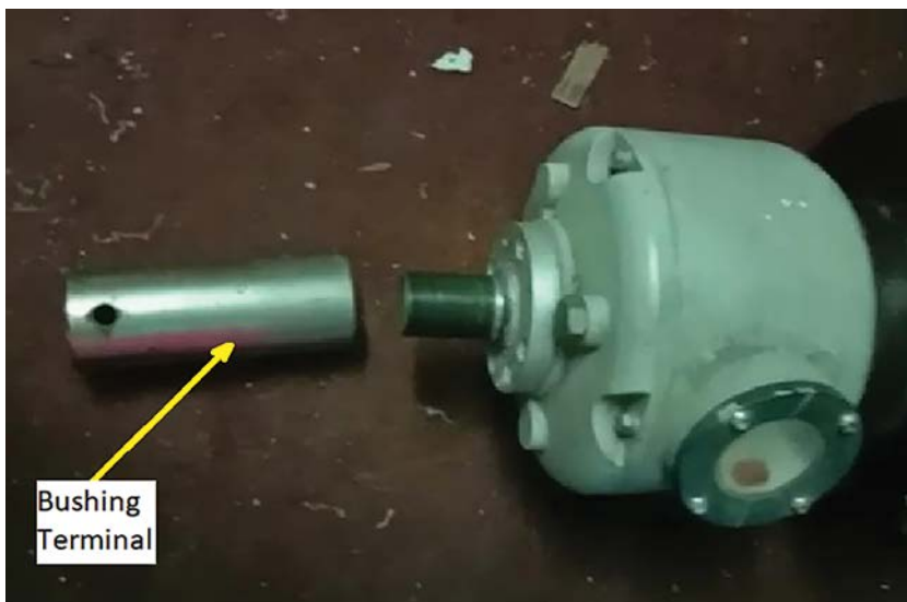
Figure 7E. Display of a bushing terminal
