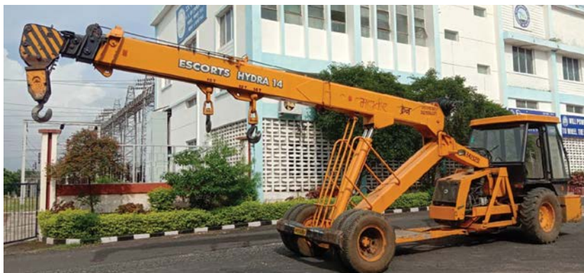
Figure 5B. Hydra Long-boom crane
