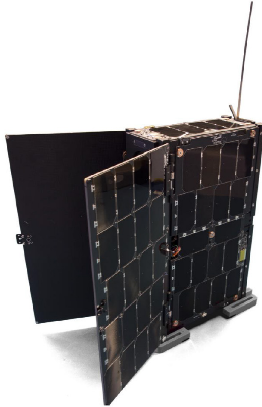
Figure 29. Integrated Corvus-BC spacecraft based on Corvus-6 6U bus. Source: [63].
