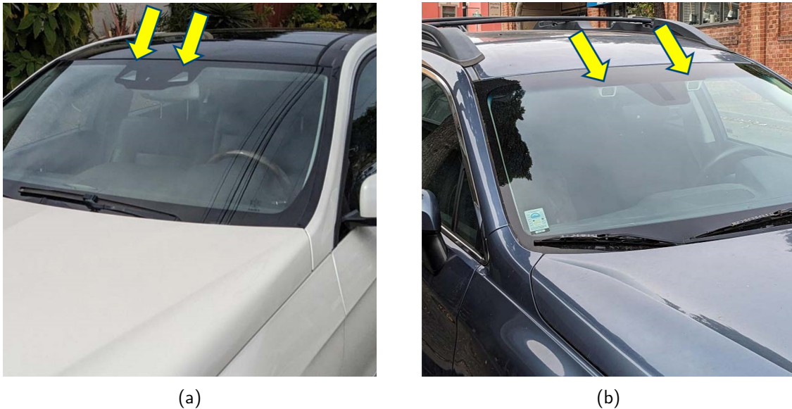
Figure 5.12. Forward looking multi-camera configurations for lane departure flanking the rearview mirror at the top of the windshield as marked with arrows on (a) a Mercedes EQE 350 and (b) a Subaru Outback.
