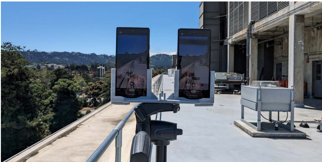
Figure 5.14. Dual camera collection at 130 m. The headlight is visible in the distance, centered between the two cameras.
