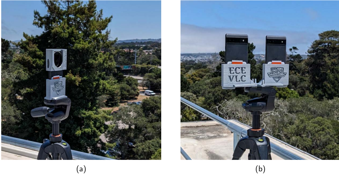
Figure 4.3. (a) Single and (b) dual mounts for collection on the roof of the engineering building.
