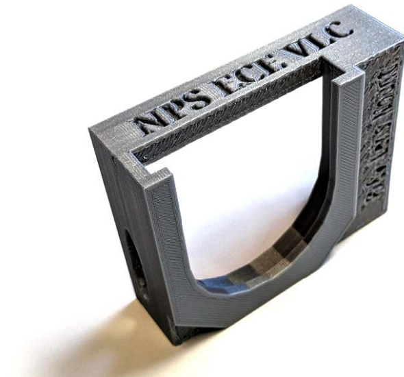
Figure D.2. A printed lens mount, one of several pieces used to fix and stabilize the Pixel 6a and filters during experimentation.
