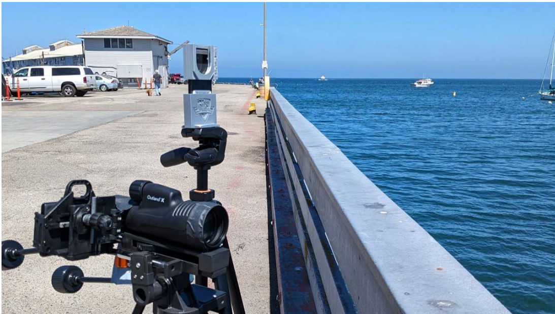
Figure 5.9. Receivers for the 1650 m experiments, with the Pixel 6a mounted to a 20× monoscope in the foreground and a Pixel 6a with no additional magnification (as used in all other experiments) in the back.
