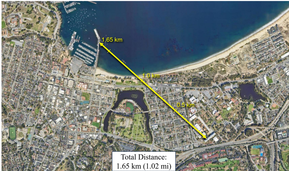
Figure 4.4. The 1.65 km test range from the roof of the engineering building to the municipal wharf in Monterey. Adapted from [122].
