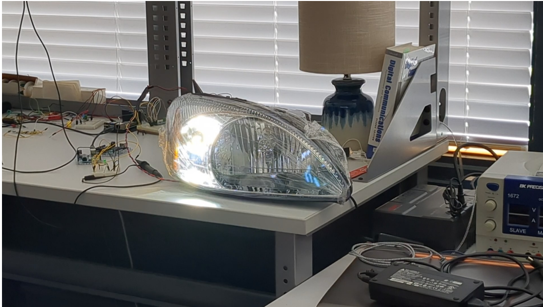
Figure B.5. Customized, controllable LED mounted in the left side reflector area of the headlight assembly.
