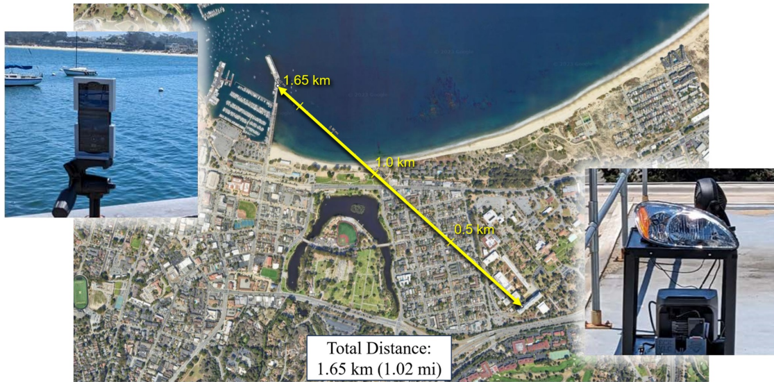
Figure 2. Overview of components used in experimentation, including the receiving Pixel 6a camera phone mounted on a tripod, the geometry of the 1650 m test over Monterey Bay, and the transmitting LED headlight. Adapted from [7].
