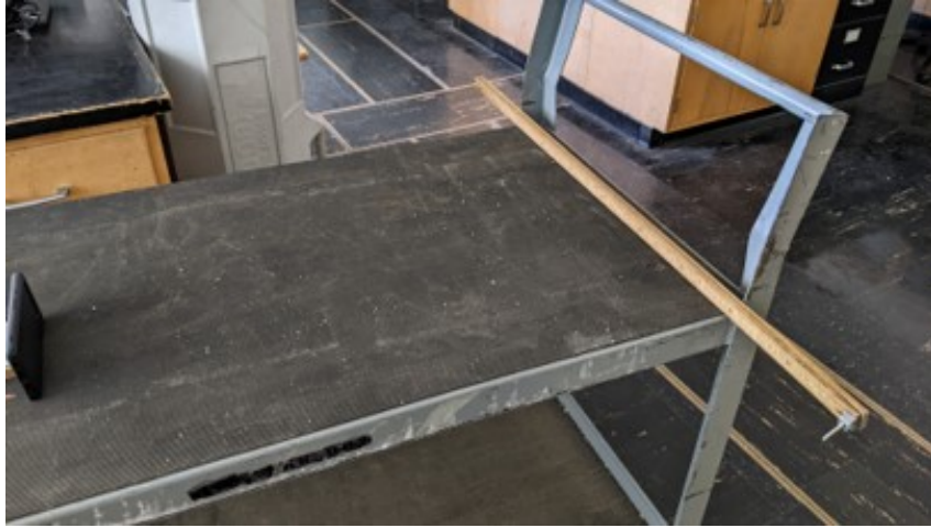
Figure 4.6. Calibrating the Pixel 6a FOV by recording a meter stick.
