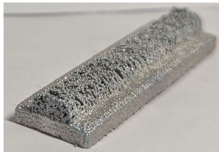
Figure 23. Sample 16: Wick PHT 0.092 ms, Jetting Frequency: 20%, Print Optimization: Off, Infill Type: Shell.
