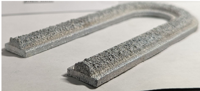
Figure 40. U-Shaped Design 3 (PHT: 0.095 ms, JF: 20%, Shell Infill).
