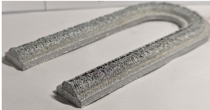
Figure 39. U-Shaped Design 2 (PHT: 0.095 ms, JF: 20%, Standard Infill).
