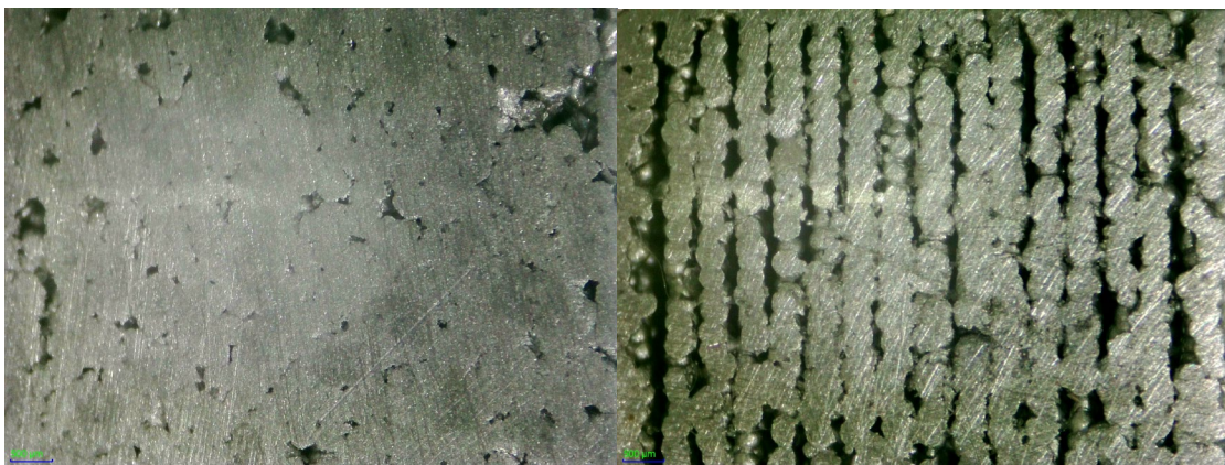
Figure 26. Cross-sections 5–6: PHT 0.100 ms, JF 10%. Standard Infill (Left) and Shell Infill (Right).
