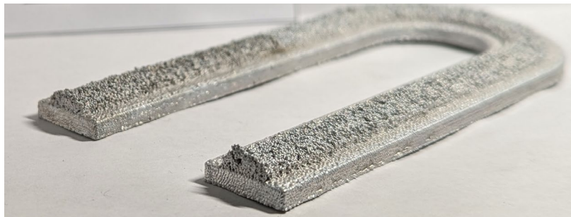
Figure 43. U-Shaped Design 6 (PHT: 0.090 ms, JF: 20%, Shell Infill).
