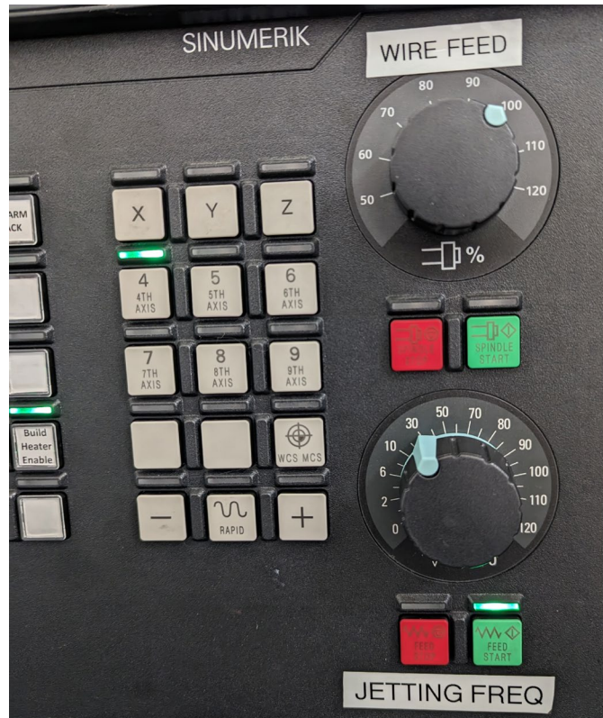
Figure 4. Operator Button Panel.
