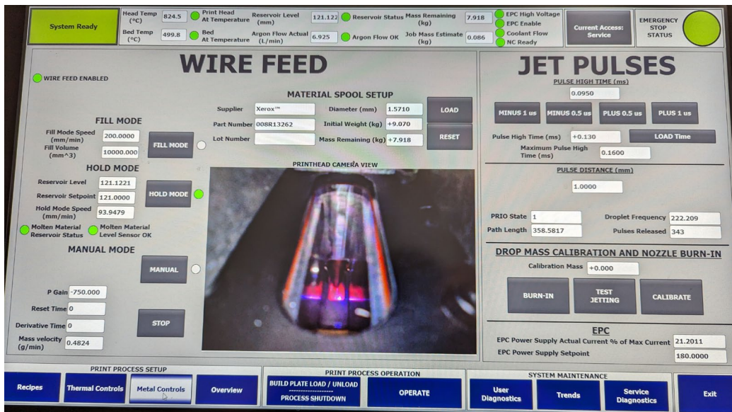
Figure 3. HMI Menu for Metal Controls.
