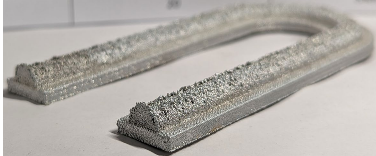
Figure 38. U-Shaped Design 1 (PHT: 0.100 ms, JF: 20%, Shell Infill).
