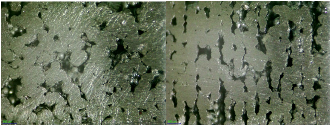
Figure 30. Cross-sections 13–14: PHT 0.090 ms, JF 30%. Standard Infill (Left) and Shell Infill (Right).
