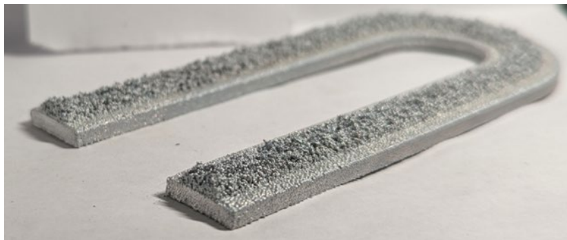
Figure 42. U-Shaped Design 5 (PHT: 0.090 ms, JF: 30%, Shell Infill).
