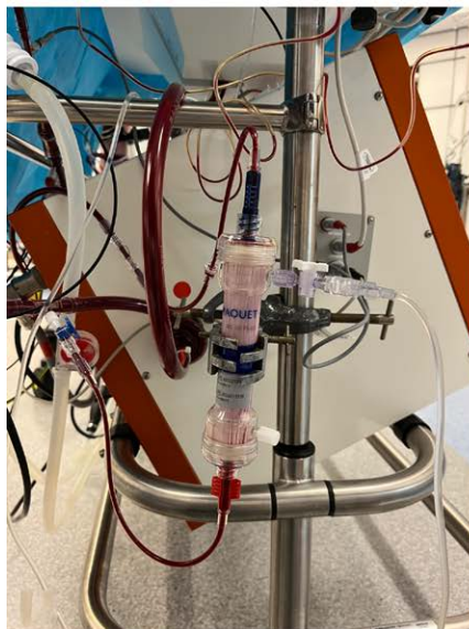
FIGURE 1. A, Setup of the CRRT by addition of a pediatric dialysis filter into the existing Liver Assist disposable set (XVIVO, Groningen, The Netherlands) for liver machine perfusion. The black interrupted line surrounds the added circuit for CRRT to the existing perfusion circuit. The perfusate inflow to the dialysis filter (B) was positioned after the arterial pump to benefit from the highest pressure in the system and to avoid the addition of an extra pump to minimize hemolysis. Perfusate outflow from the dialysis filter was returned to the outflow line coming from the liver reservoir to avoid shunting of hypoxic perfusate. Drainage of ultrafiltrate from the dialysis filter was facilitated by a roller pump (C). The roller pump speed was manually adjusted on the basis of the osmolarity level of the perfusate, which is mainly affected by the sodium, glucose, and urea levels. The substitution fluid inflow was positioned after the dialysis filter to obtain an ultrafiltrate composition that can be used for analyses of glucose and lactate values in the ultrafiltrate. The substitution fluid was connected to a separate roller pump. The speed of the substitution fluid infusion was matched to the ultrafiltrate flow to maintain a stable perfusate hematocrit. CRRT, continuous renal replacement therapy.
