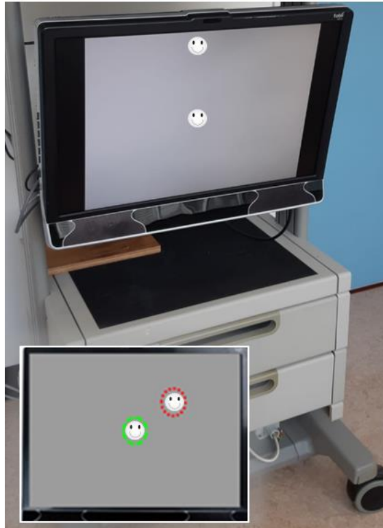
Figure 5.1: EMPP set up with a 24-inch display monitor integrated with an infrared eye-tracking device and a height/viewing angle adjustable surface housing. The inset picture shows an illustration of the smiley fixation target (circled with green dotted lines) and a peripheral smiley stimulus (circled with red dotted lines).
