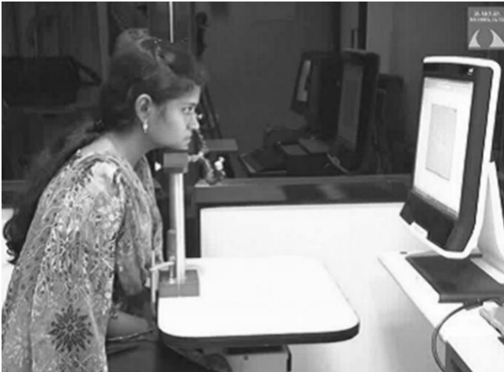
Figure 3.2: Illustration of a participant sitting in front of the Eye Movement Perimetry (EMP) test set up consisting of an eye tracking device integrated into a Thin Film Transistor (TFT) monitor.
