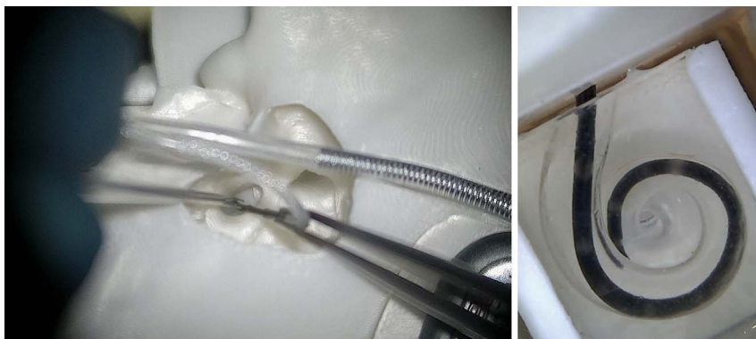
FIG. 1. Left: View through the surgical microscope showing the temporal bone model and mastoidectomy, and the black dummy electrode array attached to the electrode lead of the implant body. Right: Photomicrograph of the scala tympani model of the same insertion, showing the partially inserted array. A small air gap (0.5 mm) decouples the scala tympani model mechanically, allowing to measure insertion forces unaffected by the promontory.
