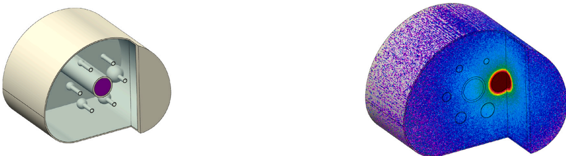
Fig. 2. FLUKA implementation of the NEMA IQ phantom (left) and an illustrative example of a 3D dose distribution from FLUKA with cartesian grid scoring (right).
