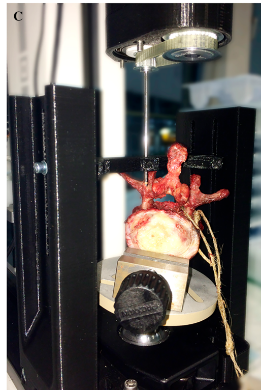
Figure 1. (A) Flowchart of overall procedure. (B) Dissected spine from thoracic vertebra T11 to L5 from individual B, left dorsal view. (C) Lumbar vertebra during trans-pedicular drilling using a motorized material testing machine (Mark-10 Force Test Stand ESM301) as previously described 14 , supplied for the present study with clinical drilling tools (ARROW OnControl Bone Lesion Biopsy System Tray).
