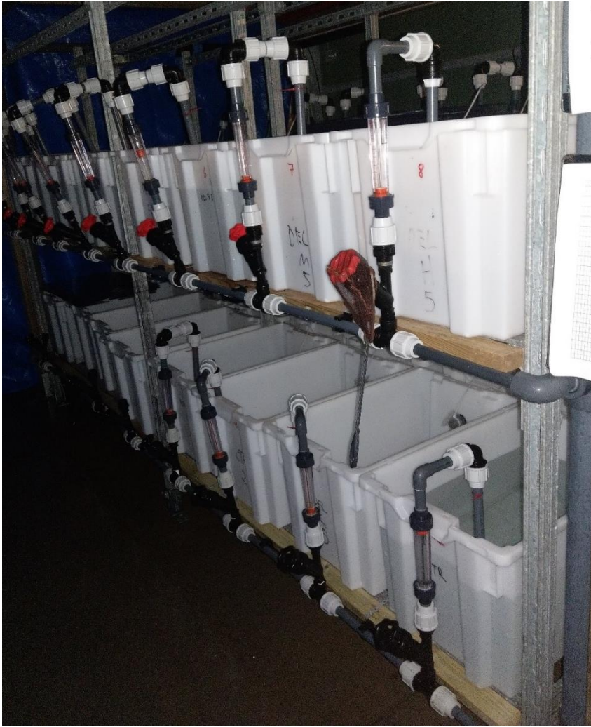
Figure S2.2: Experimental set up of shrimp exposure with 45 l tanks and flow through systems.
