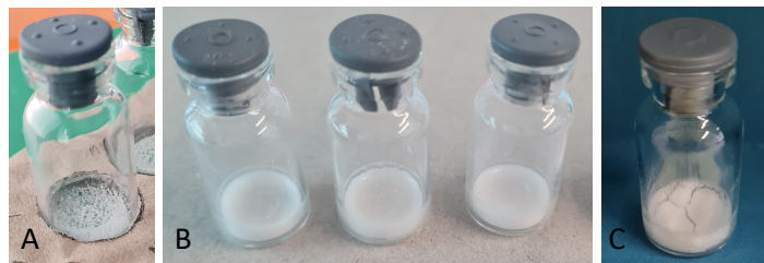
Figure 1.14: Examples of lyophilized drug product cake appearances. A) shows an example of total collapsed cake or meltback. B) shows no sign of collapse or cracking. C) shows an example of cracked cake. Photo: Cindy Zhang.
