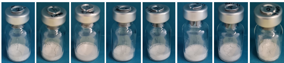
Figure 5.7: Photos of cracked lyophilized cakes due to issues during the freezing process. Photo: Cindy Zhang.
