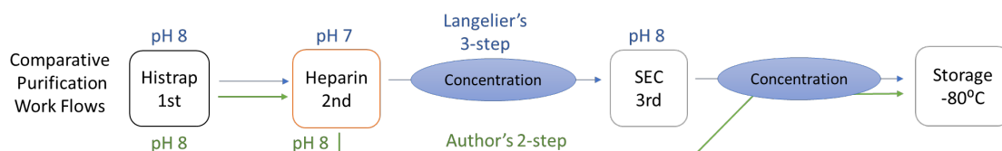
Figure 8. Purification workflow. A schematic comparison of the 3-step (Langelier et al. [16]) and 2-step (Author's present work) PARP1 purification protocols.
