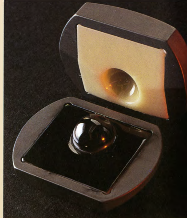
Professor Vijay Goel and his colleagues are testing this artificial spinal disk for the company that designed and manufactured it. The UI researchers measure factors such as range of motion, load bearing, and wear and tear. If the implant meets its designers' expectations, it could be used in human spine patients soon.
