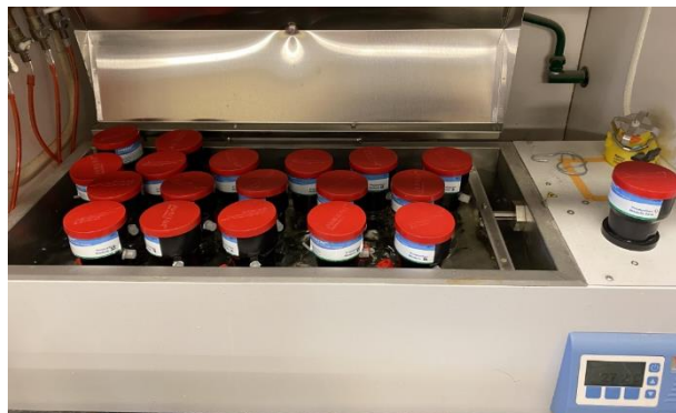
Sealed digesters in the agitating water bath
