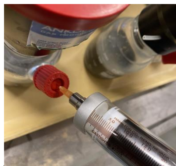
Sampling gas from digester
