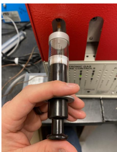
Injecting gas sample into the GC
