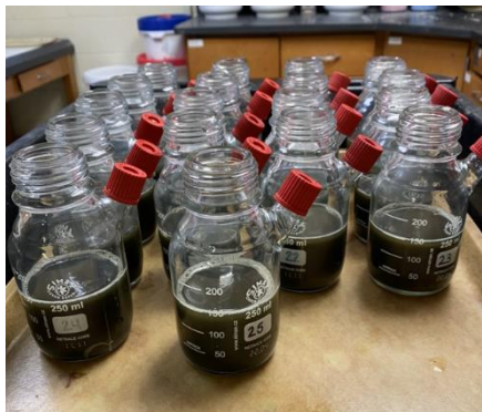
Digesters loaded with substrate, inoculum, and DDW before topping with ANKOM modules
