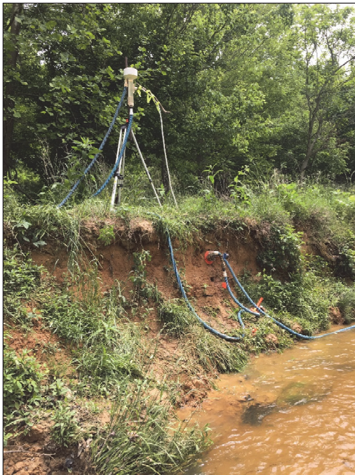
Figure 2. A mini-JET device deployed on a streambank in Millstone Creek, North Carolina, to characterize its erodibility. In this setup, a constant pressure head tank is being used to drive the impinging water jet.
