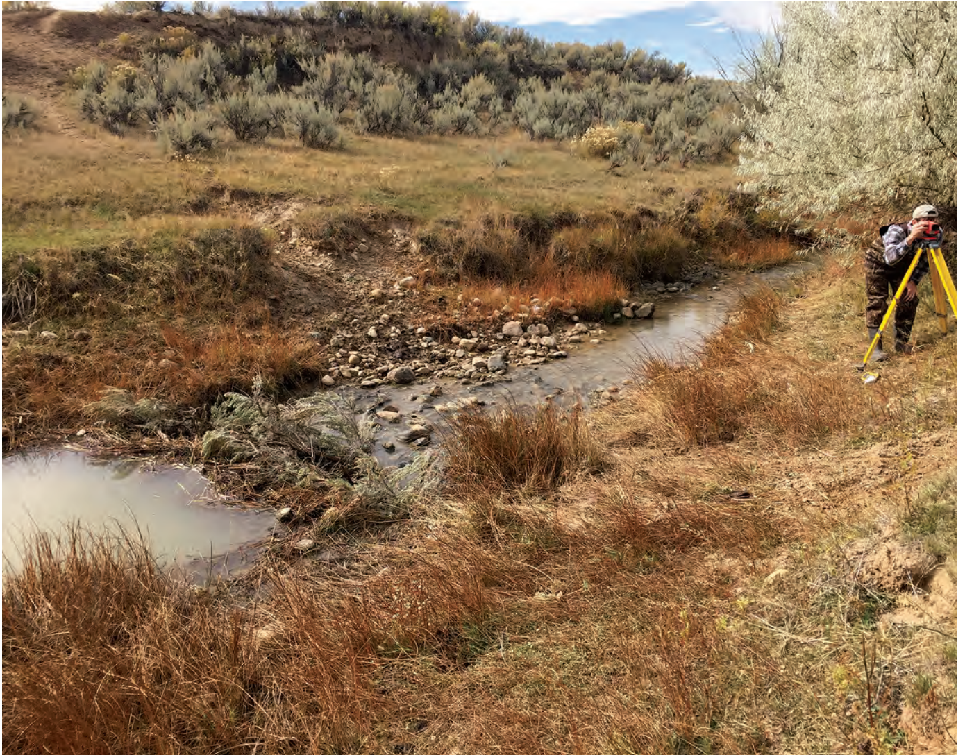
Figure 6. Photograph showing a U.S. Geological Survey hydrologist (from the Wyoming-Montana Water Science Center) using surveying equipment to measure elevations on Muddy Creek near Baggs to ensure accurate data collection. Photograph by Cheryl A. Eddy-Miller, U.S. Geological Survey, 2018.
