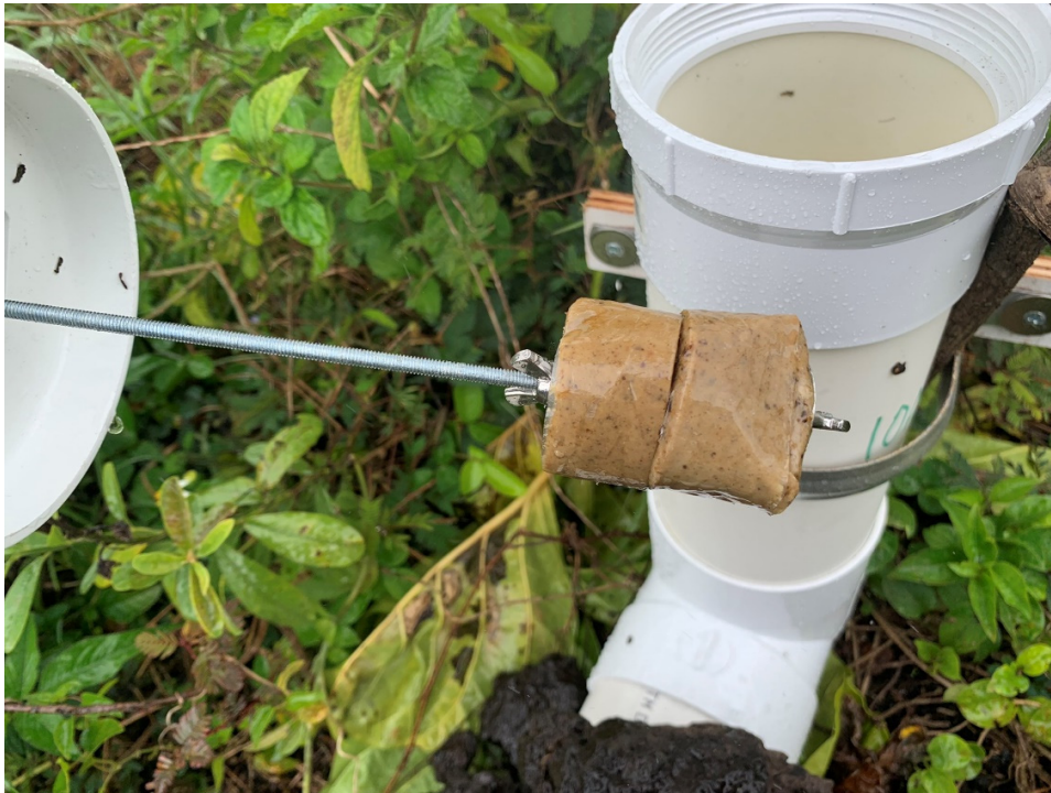
Figure S3 Prototype Bait Station, PVC “L” shaped design, deployed at the field sites.
