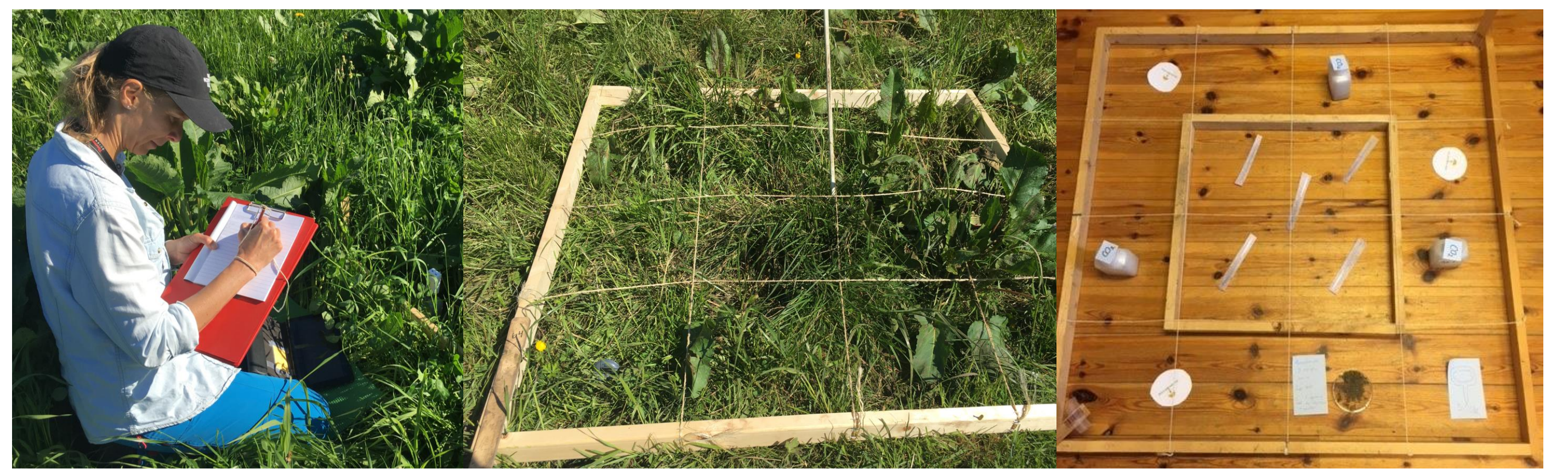
Fig.2. All tests were done within and from soil close to a frame of 1m x 1 m, in three places at each field. Five bait lamina stick, for measuring feeding activity, were placed in the middle of the "frame area".
