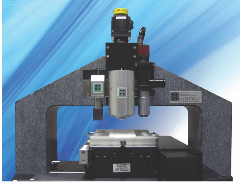
Figure 6.1 Image of Triboindenter with Omniprobe (center) used for a nanoscratch test (image taken from hysiton.com).
