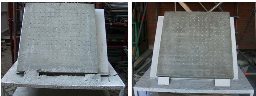
Fig. 6. Settled dust: without DustBubble (left) and with DustBubble (right).
