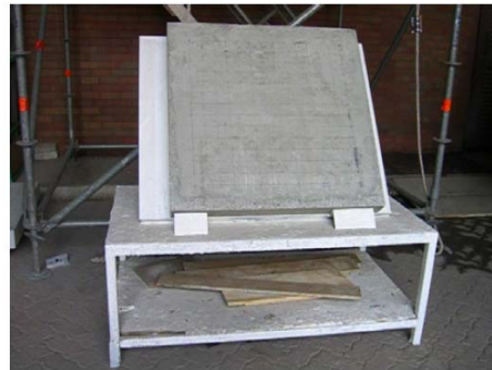
Fig. 4. A support for holding concrete blocks.
