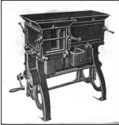
Figure 6: An example of H. S. Palmer's first cast iron concrete block machine. Eno, 75.
