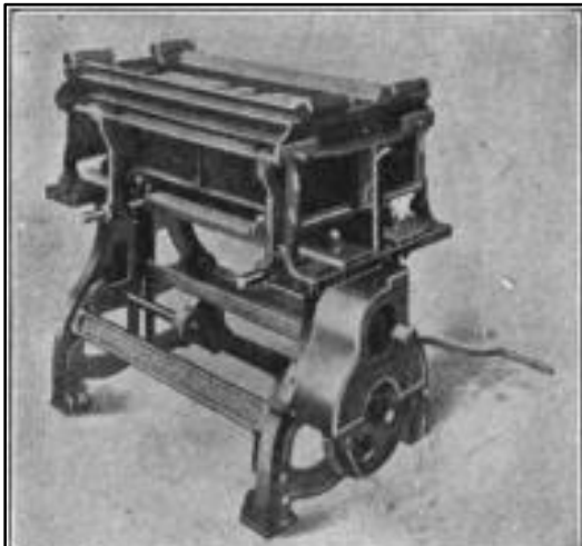
Figure 7: An H. S. Palmer machine in the closed position. The Palmer machine is an example of a side mount machine. Homer A. Reid, Concrete and Reinforced Concrete , The Myron C. Clark Pub. Co., New York, 1908, 869.
