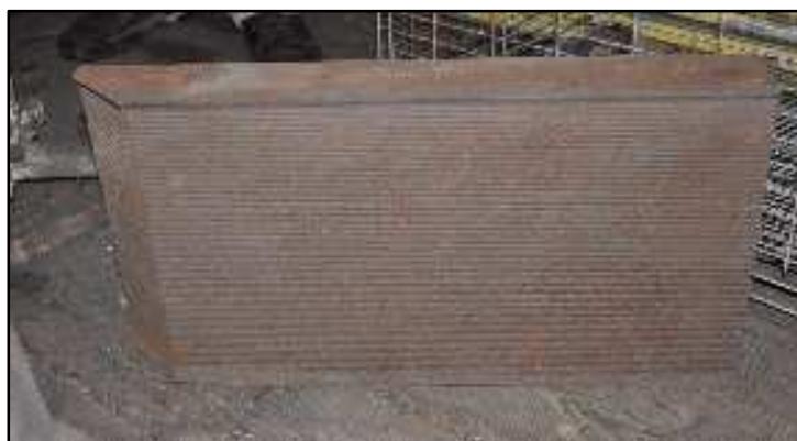
Figure 16: The picture to the left is a cast iron tool-face mold manufactured by the American Hydraulic Stone Co. Photo by James Hall
