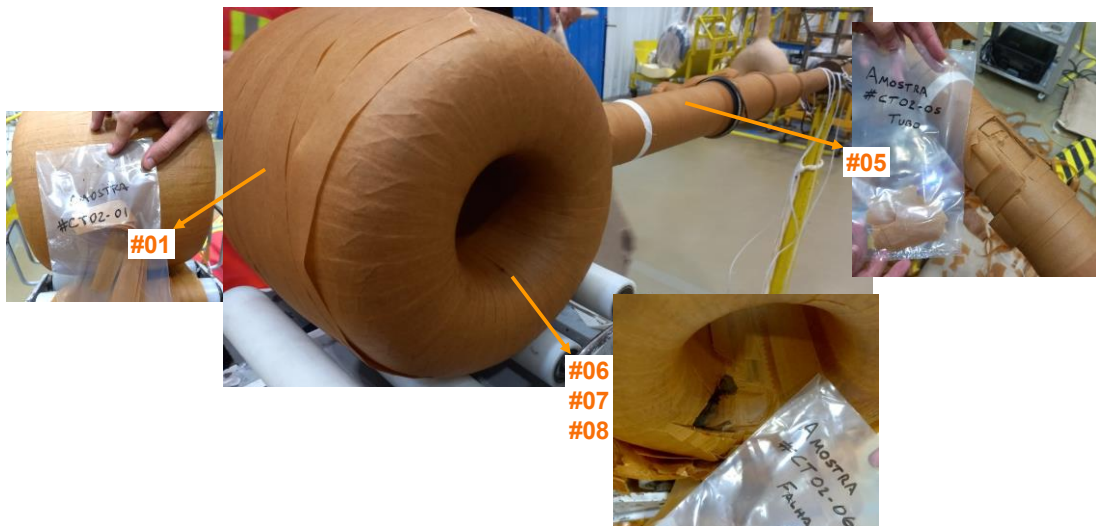
Figure 55 – Active part of the sample CT02 – Identification paper samples withdrawn for degree of polymerization and SEM-EDS analysis.
