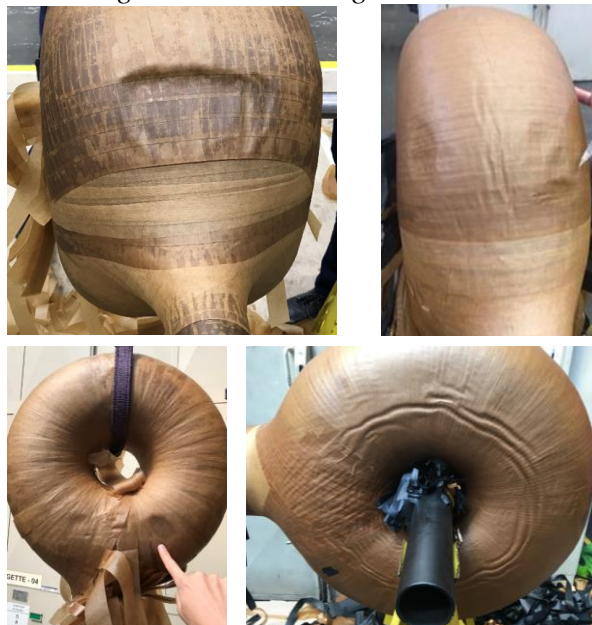
Figure 5 – Examples of geometrical insulation system defects associated with partial discharges detected during routine tests.
