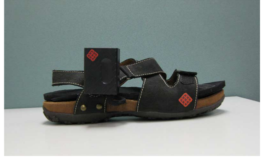
Fig. 5. Prototype of the in-shoe plantar pressure measurement system.
