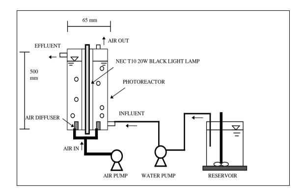
Figure 1. Sketch of a continuous flow photo-reactor system
