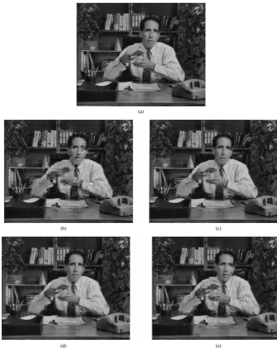
Fig. 6. Reconstructed frame 16 of the sequence Salesman at 0.1 b/pixel. (a) Original. (b) Fixed temporal-length 3-D DCT coding. (c) Proposed 3-D DCT coding using ABF. (d) Proposed 3-D DCT coding using MAD. (e) MCTC technique.
