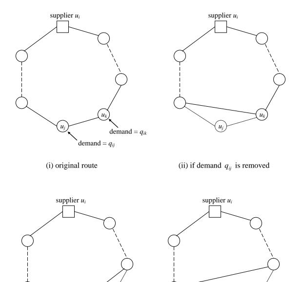
Figure 2. The situation when demands  $q_{ij}$  and  $q_{ik}$  are removed from the route
