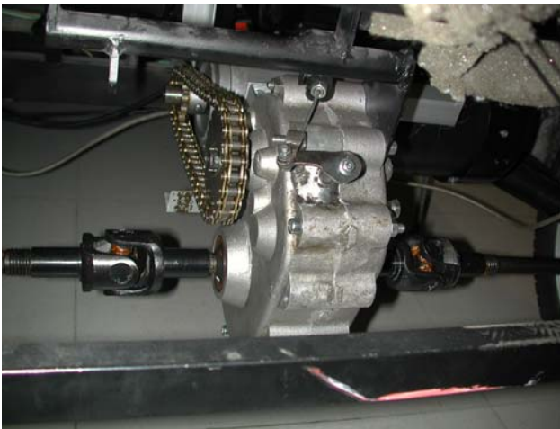
Fig 5.7: Gear and universal joint of the EV
