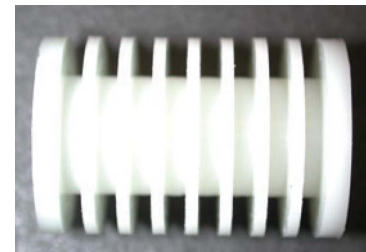
Fig. 15. Bobbin for the igniter transformer.
