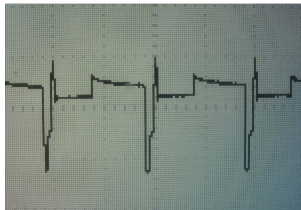
Fig. 12: The voltage of motor when O1 and O4 turning on (5V/div, 1ms/div)
