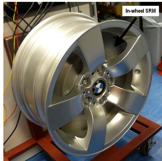
Fig. 3 Prototype of the in-wheel SRM
