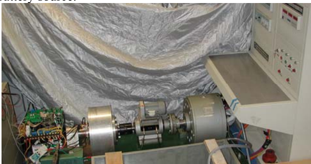
Fig. 11: Experimental direct driving system for EV
