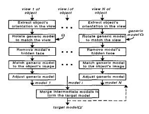
Figure 1. Flow of the Model Synthesis Process
